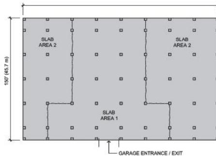
On the middle-level parking deck, the owner noticed potholes, unevenness, and cracking. The deck plan shows where concrete delamination or spalling was discovered: 60% in Slab Area 1 and 10% to 20% in Slab Area 2. The deterioration pattern suggests vehicles tracked deicing salts into the garage, which corroded the embedded reinforcement where drivers most often parked. All graphics courtesy of ACI
