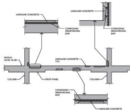
Several types of concrete deterioration were observed: delamination and spalling of the driving surface and bases of columns in areas adjacent to steel reinforcement, and cracking.
