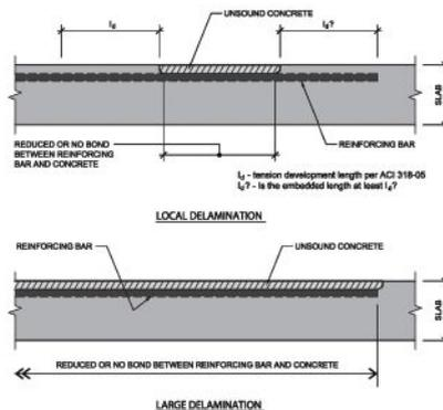
Based on the significant amount of top surface deterioration in Slab Area 1, the reinforcing bars were conservatively judged to be debonded from the concrete and therefore structurally ineffective. The concrete columns had only small localized deterioration, and were determined to be structurally sound.
